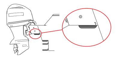
The transducer transom bracket can be mounted inside or outside of the jackplate by drilling through the jackplate and then running bolts through the hinge hole in the side of the bracket into the jackplate. The illustration above shows the transom bracket mounted inside the jackplate.
