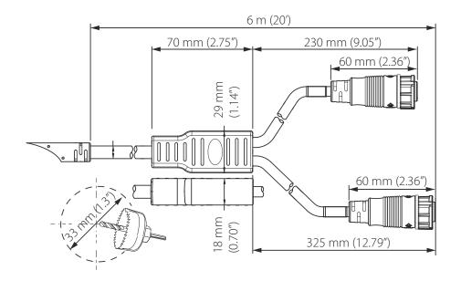
A 33mm (1.3") diameter hole is recommended for cable clearance.
